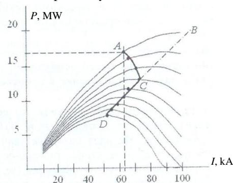
Fig. 1. Electric characteristics of the ore-heating furnace
